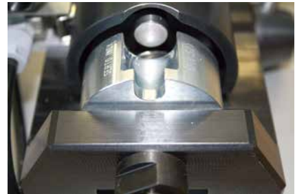
rotatable tool drum for up to five sizes
